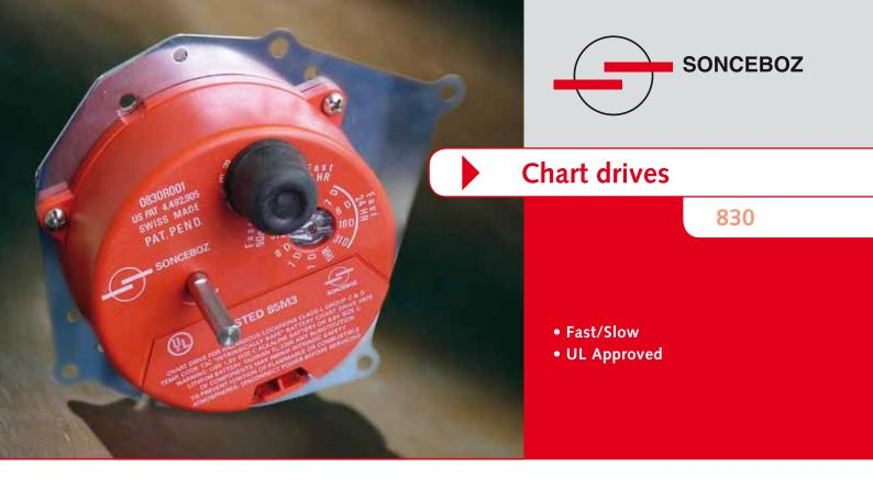
This standard chart drive offers accuracy and reliability for precision measurements. The quartz movement concept provides robustness, and it was design to operate into a temperature range of -40° F up to +140° F. The universal mounting plate makes it easy to install into all commonly use recorders.
